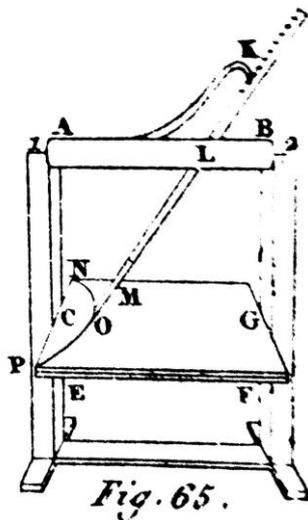
The sketch of the lens-cutting machine<sup>60</sup>
